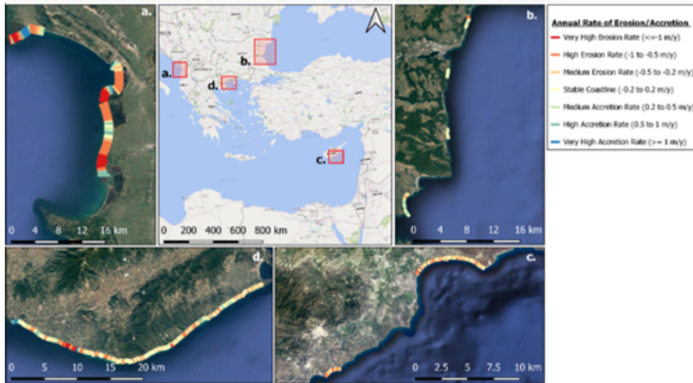
Figure. Annual rate of shoreline movement in the HERMES project study sites; a. Study sites of Albania, b. Study sites of Bulgaria, c. Study sites of Cyprus, d. Study sites of Greece.
